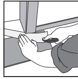
[2] Undercut doorjamb for a professional fit.
